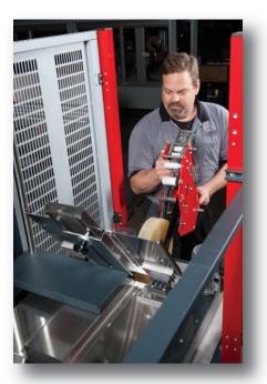
The CE-10's hinged case hold down plate allows for easy tapehead removal. The case erector's open design eliminates overhead cross members providing easy access for planned maintenance.
