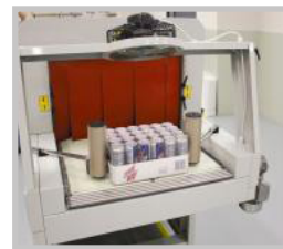
Closure rollers to flatten film against package
