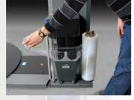
Loading stretch film is fast and easy. Just open the hinged door, pull the film tail through, and close the door. Power is automatically disconnected when the door is opened.
