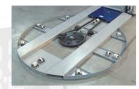
Structural steel plate and tube is used to provide a robust and durable base. Soft-start rotation prevents unstable loads from toppling when cycle begins.
