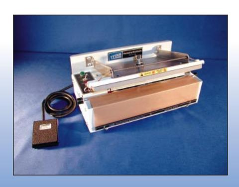
The *Titan TM Electro-Sealer TM 300*Series are high production thermoplastic bag sealers offering manual and semiautomatic settings.
