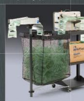
Produces continuous strips of air pillows with EZ-Tear™ Perforations for easy handling and effortless pillow separation
