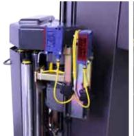
Kit includes second load height photo cell for additional turntable
