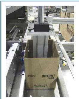
Compression ensures tight, secure seals on the widest range of case sizes and styles: RSC Regular Slotted Case CSSC With Meeting Minors RSC with 5th Panel Partition AFM All Flaps Meeting FOL Full Overlapping Flaps RSC with Reversed Glue Flaps
