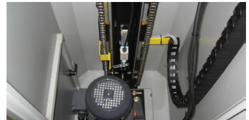
Inside the tower, dual ANSI chain and cable track are used for smooth carriage movement. The Sentry uses no-maintenance AC motors with VFD.
